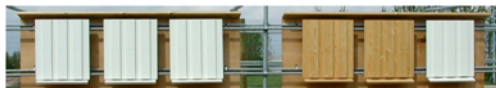
Figure 1. Test racks at the field test area of the Danish Technological Institute. Immediately after installation.
